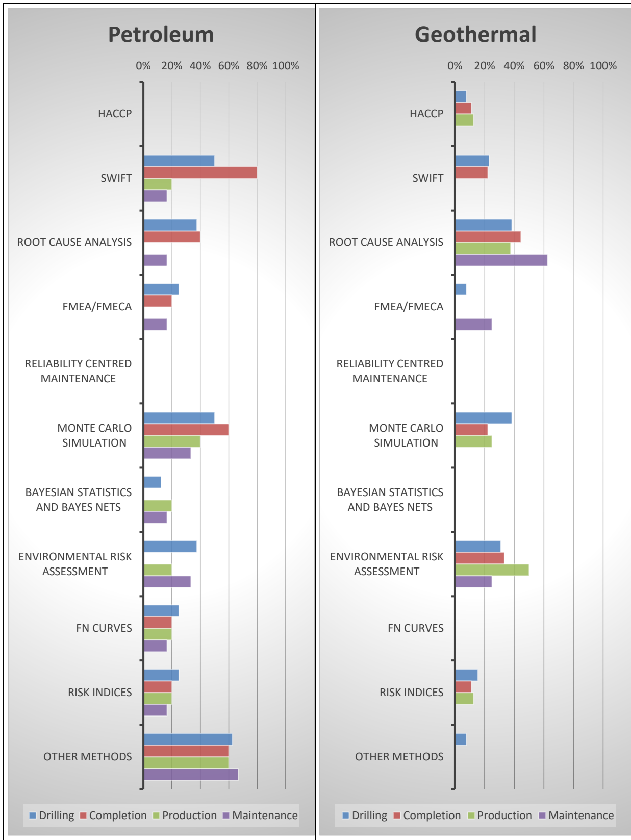
Figure 5-22 a) Overview of methods petroleum respondents used for risk evaluation, broken down on well phases, and b) Overview of methods geothermal respondents used for risk evaluation, broken down on well phases
