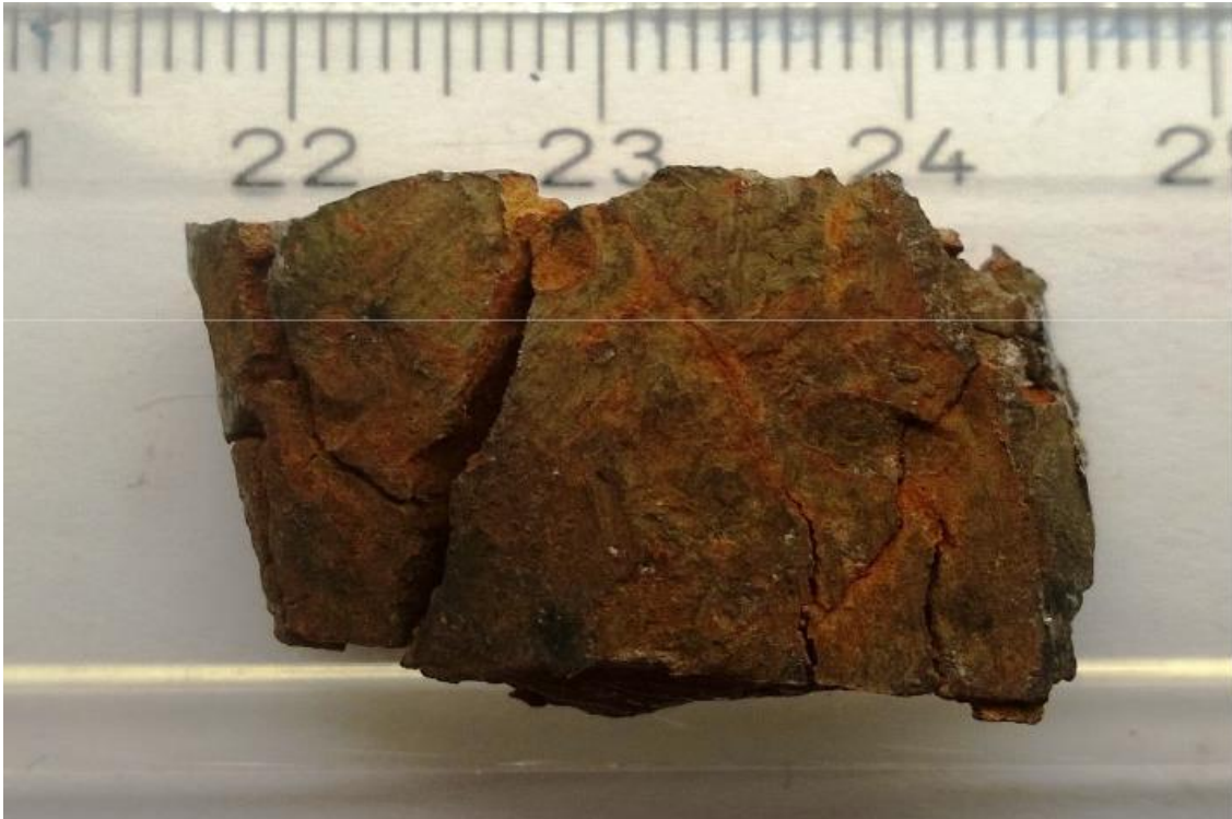
Figure 2.2.1. Material from either liner or casing in the IDDP-1 well. Retrieved during flow testing of the well (Photo from A. Einarsson).
