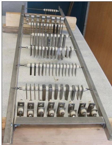
Figure 2.1.1. Picture taken of the material test rack for testing in the IDDP-1 well in the Krafla area in NE Iceland. Specimens were both stressed (u bend specimens) and unstressed, welded and not welded (Karlsdottir et al., 2015)
