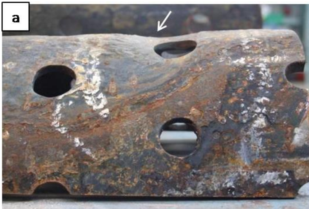
Figure 2.2.2. Retrieved part of liner from the KJ 39 well in Krafla. Severe damages due to uniform corrosion. No corrosion products detected.
