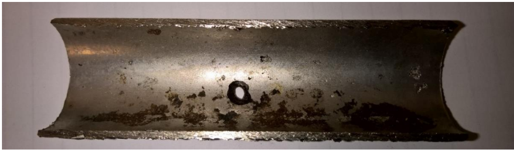
Figure 2.3.1. Pitting corrosion on the inside of a pipe of stainless steel type AISI 316. (Photo Thorbjornsson).
