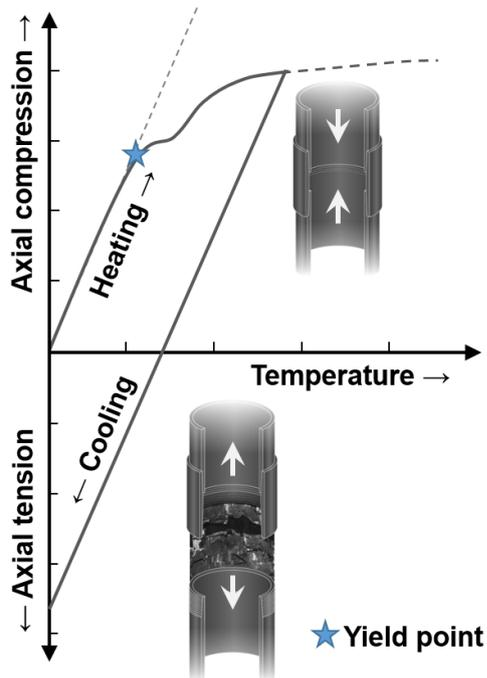
**Figure 1. Concept diagram for the failure mechanism where axial tension is generated subsequent to strain that formed in compression (adopted from a diagram by Rahman & Chilingarian, 1995).**
