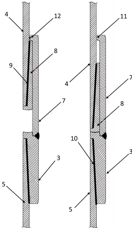
**Figure 3. Concept drawing revealing the main principles of the flexible couplings. On the left is the coupling shown in open mode, on the right in closed mode. As shown the casing segment nr. 4 slides downward during warm up together with a sled nr. 8 and at given distance the coupling close by pressing the sled nr. 8 into a seat in the coupling lower part nr. 3. (Patent application no. 050129 – Thorbjörnsson 2015).**
