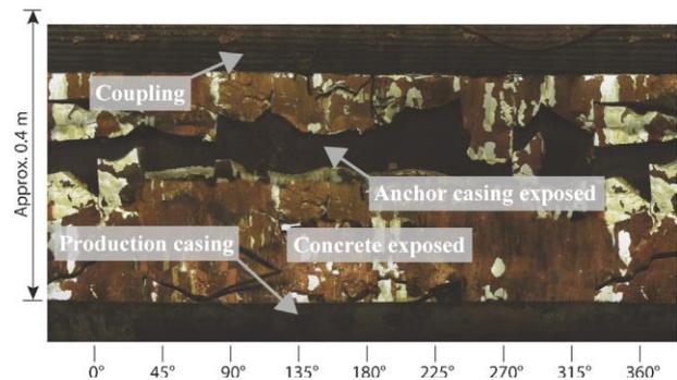
**Figure 2. Coupling rupture as a result of quenching of IDDP-1 at approximately 300 m depth (Kaldal, et al., 2016).**
